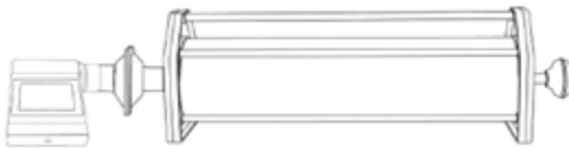
Figure 3: Micro Spirometer connected to a 3L syringe
