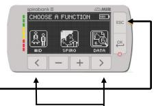
Use the left & right arrow buttons to scroll up and down through configuration menu.
