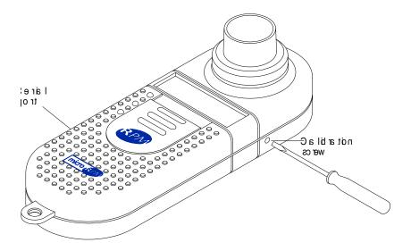
To calibrate the MicroRPM, connect the water manometer as before, filling the syringe to obtain the required negative pressure. To change the calibration, slowly turn the calibration screw in a clockwise direction until the same value is displayed on the MicroRPM.
