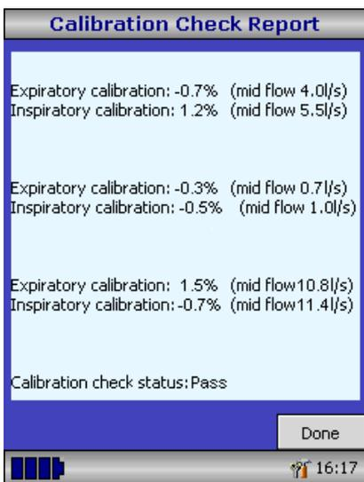
The calibration error for expiration and inspiration at each flow rate are displayed. The calibration error should be less than 3.5%. If a greater error is shown, repeat the procedure ensuring that the syringe is emptied and filled in a smooth manner without jerking the handle. If an error greater than 3.5% is still shown, inspect the turbine transducer and clean if necessary.
