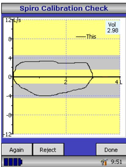
Connect a 3-liter syringe to the transducer with the minimum of adapters and empty by pushing the handle fully in.
