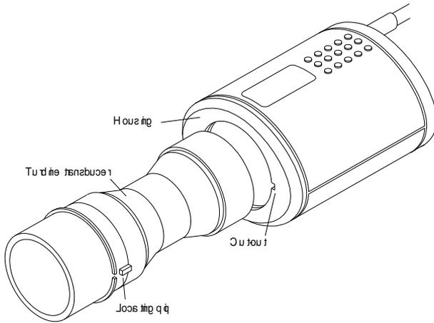
**CAUTION:** Do not attempt to wash or immerse the MicroLab transducer housing in water or cleaning fluid, as there are electronic components inside that will be permanently damaged.
