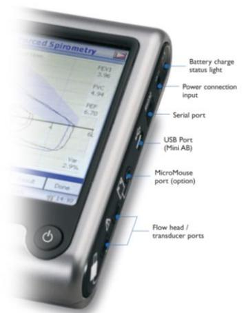
Please ensure that the turbine transducer is plugged in to either of the two sockets on the right-hand side of the instrument.
